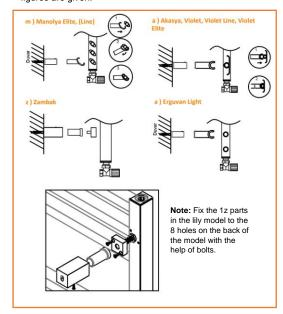
**4)** Fix the assembly parts with the fixing bolt by interlocking them.
